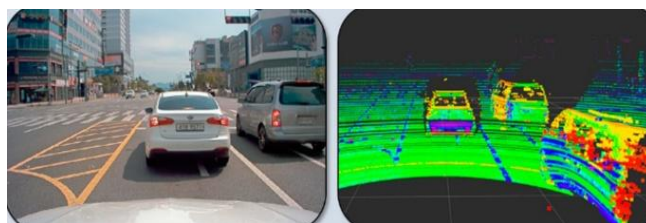
Figure 7. Comparison of vision-based and LiDAR-based obstacle detection in urban driving scenario
