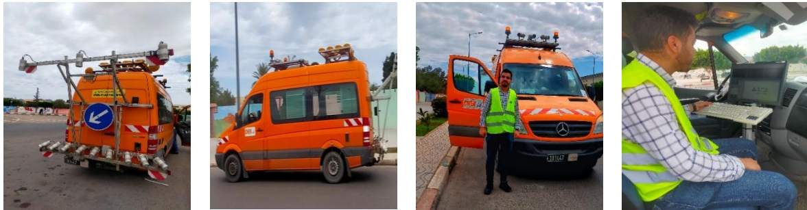
Figure 3. Pavement inspection vehicle equipped with multifunctional pavement assessment system (SMAC)
