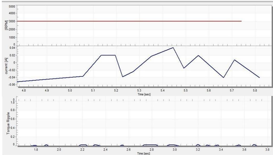
Figure 13. DTC-CBSVM twelve switch NPCI PMSM drive output at 3000 rpm
