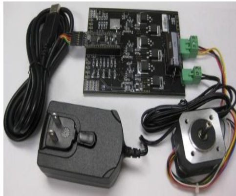
Figure 10. Experimental design of DTC-CBSVM twelve switch NPCI PMSM drive
