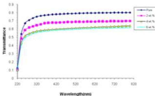
Figure 2. Effect of magnesium oxide nanoparticle on optical transmittance of (PVP-CMC) blend
