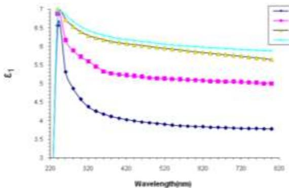
Figure 8. Variation of real part of dielectric constant with photon wavelength
