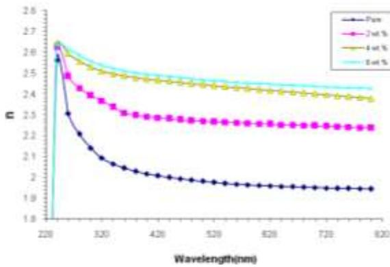
Figures 6. Variation of refractive index with photon wavelength for different concentration of MgO nanoparticle
