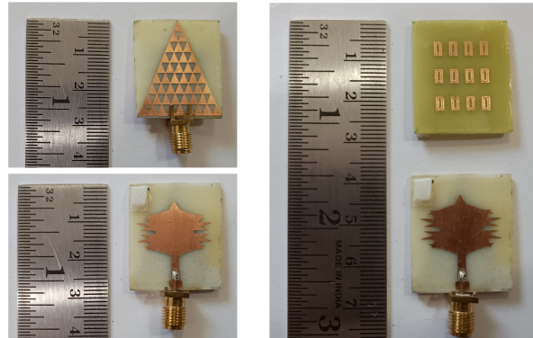
Figure 3. Overview of the proposed asymmetrical star-shaped fractal antenna with metasurface and fractal ground
