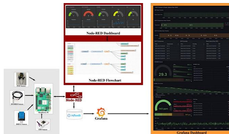
Figure 2. System architecture for IoT water quality monitoring
