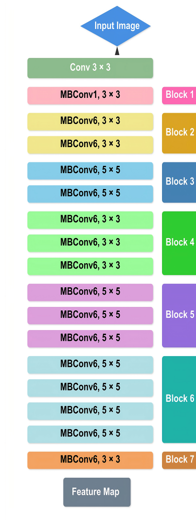
Figure 3. EfficientNet-B0 architecture with MBConv blocks and SE attention mechanisms for cocoon quality classification
