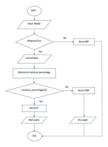
Figure 4. Flowchart of the prototype automatic waste separation system methodology
