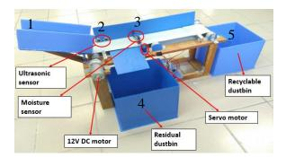
Figure 3. The prototype automatic household waste separation system
