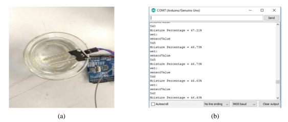
Figure 6. (a) Measurement of resistance value of water, (b) Resistance value ( $\Omega$ ) and percentage of moisture content of water (%) from Arduino software
