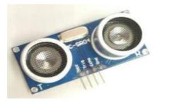
Figure 1. Ultrasonic sensor
