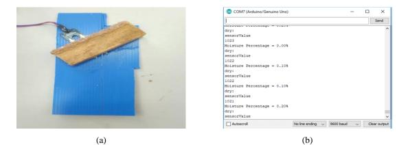
Figure 7. (a) Measurement of resistance value of wood, (b) Resistance value (Ω) and percentage of moisture content of wood (%) from Arduino software
