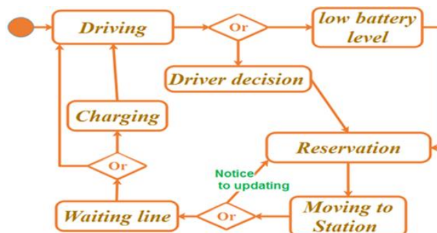
Figure 1. Flowchart of EV charging transition state
