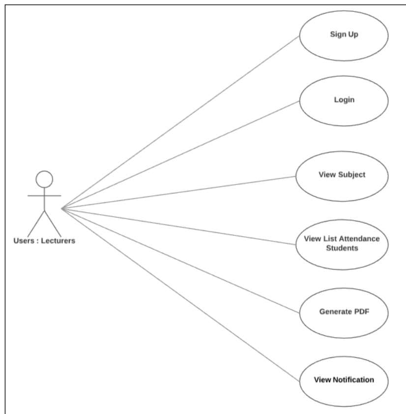
Figure 1. City i-Tick use case diagram
