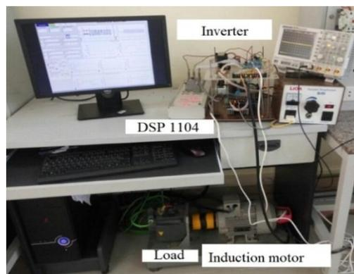
Figure 3. Photo of experimental setup
