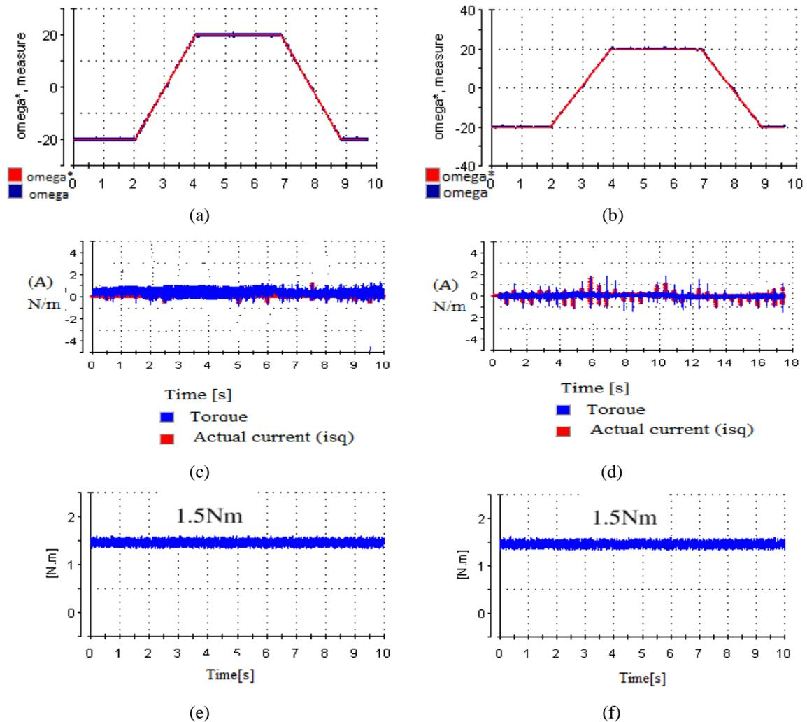
Figure 5. Torque and speed responses, (a) Speed response PCC-FOC, (b) Speed response PI-FOC, (c) Torque response with no load PCC-FOC, (d) Torque response with no load PI-FOC, (e) Torque response with load PCC-FOC, (f) Torque response with load PI-FOC
