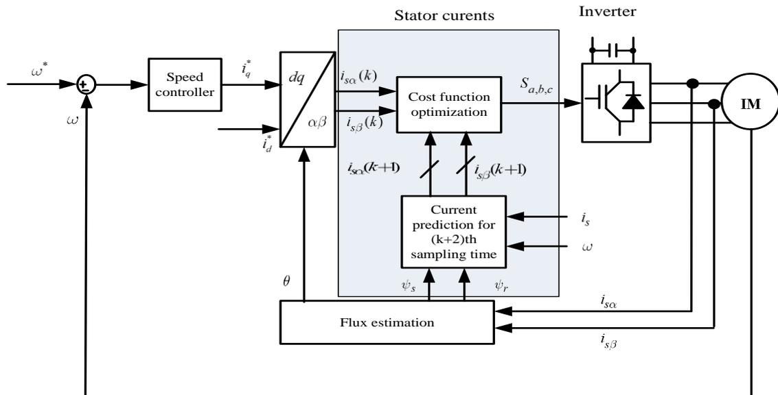
Figure 2. Block structure of the stator current controllers with predictive current controller
