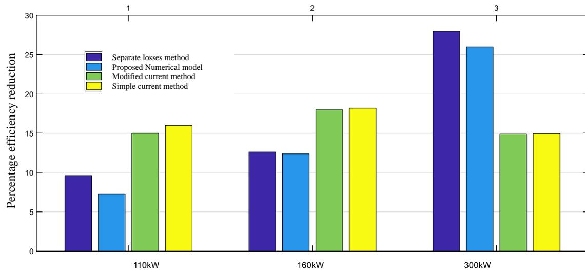
Figure 4. Comparison of experimental results of each motor with the numerical results
