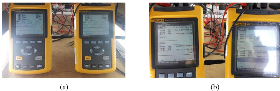
Figure 2. Recording behaviour monitored by Fluke 43B, (a) Instantaneous sampling, (b) Continuous data
