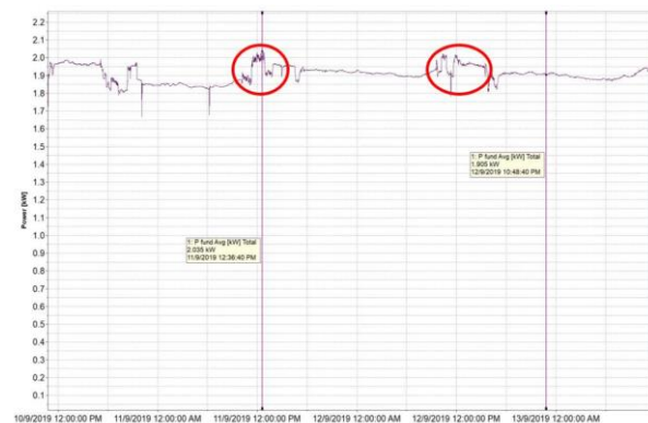
Figure 2. Power consumption measurement of the 5G testbed for four days
