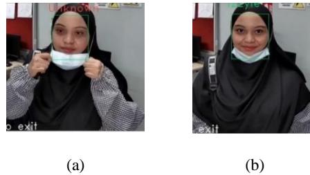
Figure 6. (a) Unknown face recognition due to non-frontal image, (b) Correct recognition using a frontal image
