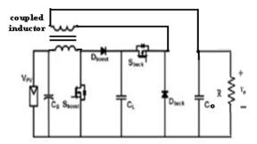
Figure 2. Boost–buck-based PV system with coupled inductor
