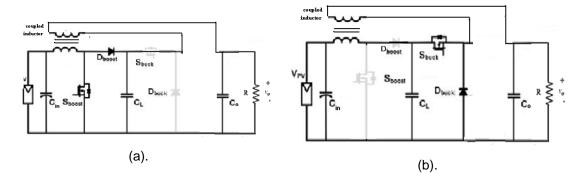
Figure 3. Operation Principle Modes: (a). Boost mode, (b). Buck mode
