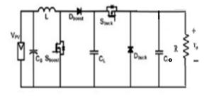
Figure 1. Boost-buck-based PV system
