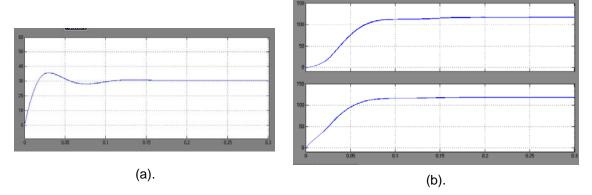
Figure 9. Boost mode of operation of converter; (a). PV panel output voltage, (b). Converter output & power in Boost mode
