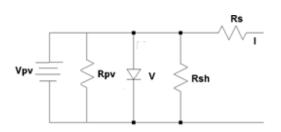
Figure 6. Solar cell model with serial and parallel resistance
