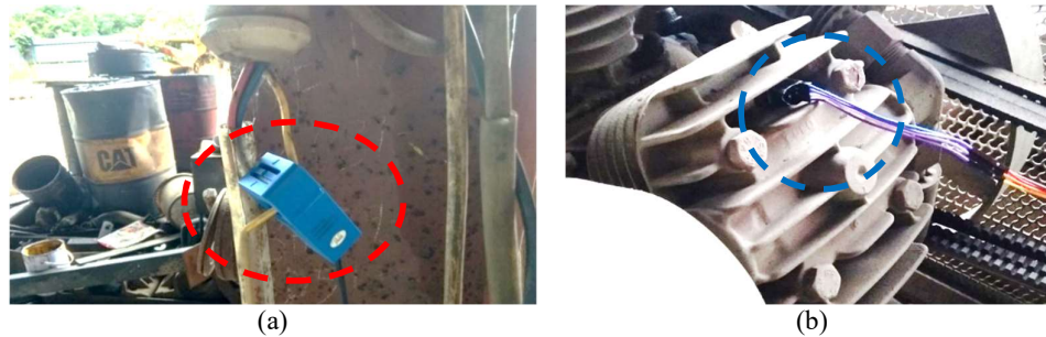
Figure 4. The placement of non-intrusive sensors on the target compressor (a) SCT-013-030 current sensor and (b) GY-906 MLX90614
