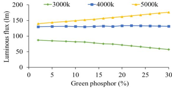
Figure 6.  $\text{Sr}_3\text{WO}_6:\text{U}$  concentration functions as the luminous flux of WLEDs
