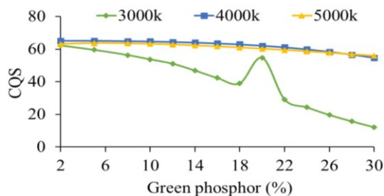
Figure 9.  $\text{Sr}_3\text{WO}_6:\text{U}$  concentration functions as the color quality scale of WLEDs
