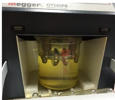
Figure 2. Photograph of the oil sample in the test chamber. The gap between the semi-spherical electrodes was 1 mm
