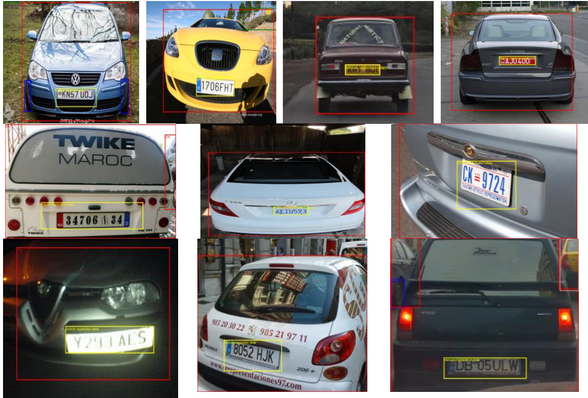
Figure 5. Vehicle level and plate level recognition
