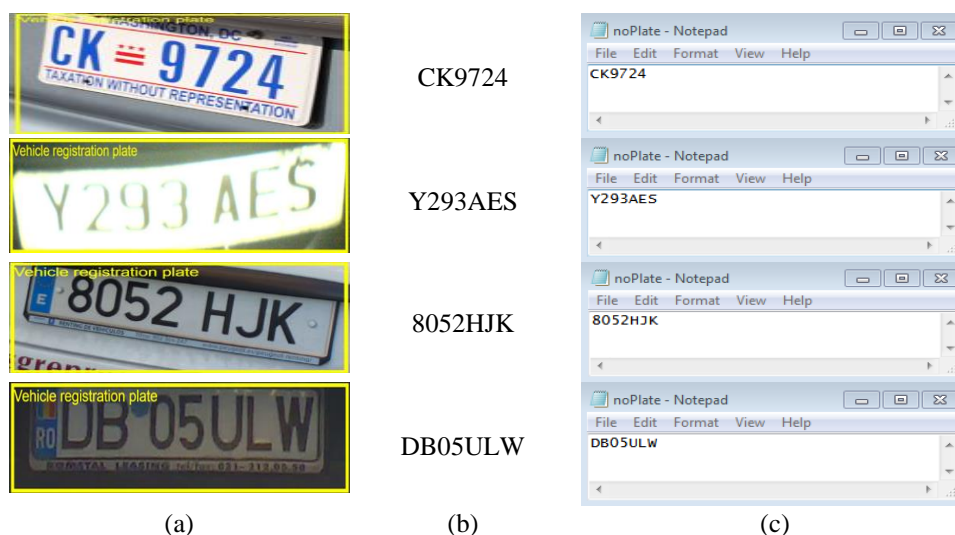
Figure 8. Character level LP recognition (a) plate level detection, (b) manual detection, and (c) character level detection (continue)
