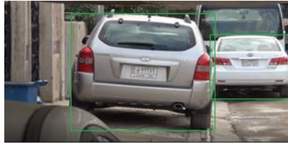
Figure 2. Sample of vehicle (car) detection with newer Iraqi license plate
