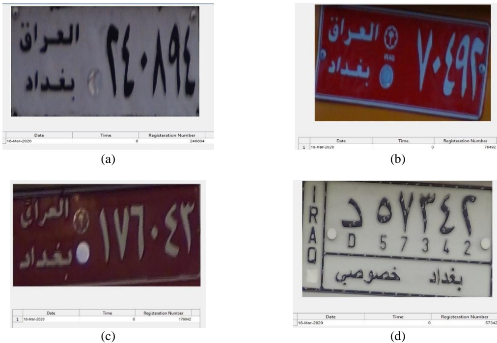
Figure 7. License plate recognition, (a) clear old private style license plate, (b) tilted captures of old public style license plate, (c) low illumination public style license plate, and (d) tilted captures of new private style license plate
