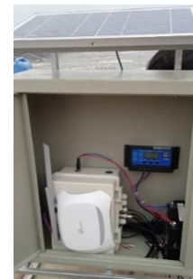
Figure 4. Monitoring cabinet (connecting sensors) meter for measuring water quality indicators
