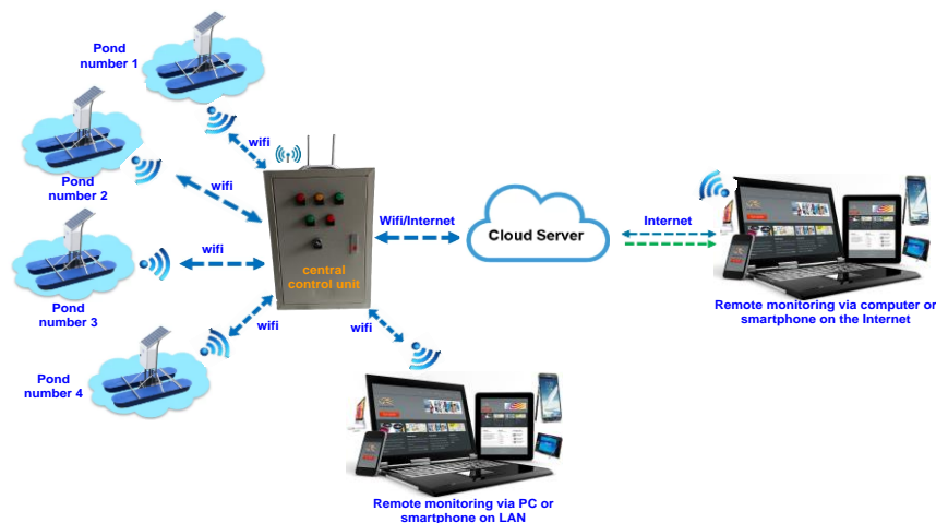
Figure 1. Model of monitoring and control system applying IoT technology
