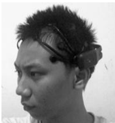
Figure 1. The test subject used Emotiv EPOC headset to record EEG data
