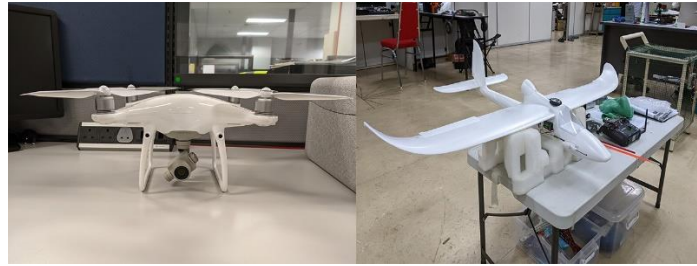
Figure 3. Multirotor drone (DJI Phantom 4 Pro V2) on the left and fixed-wing drone (Skysurfer X8) on the right
