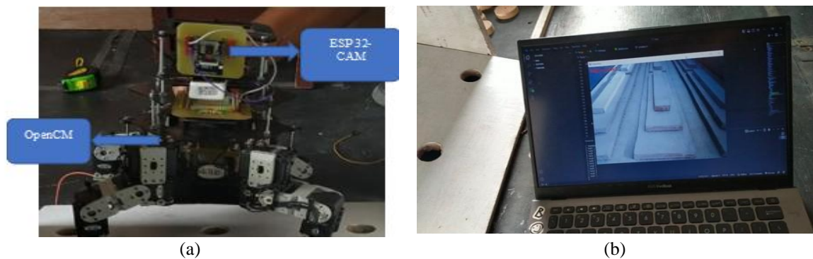
Figure 5. Test preparation configuration; (a) position of Esp32 CAM on OpenCM 9.05 robot and microcontroller and (b) position of laptop with Python programming
