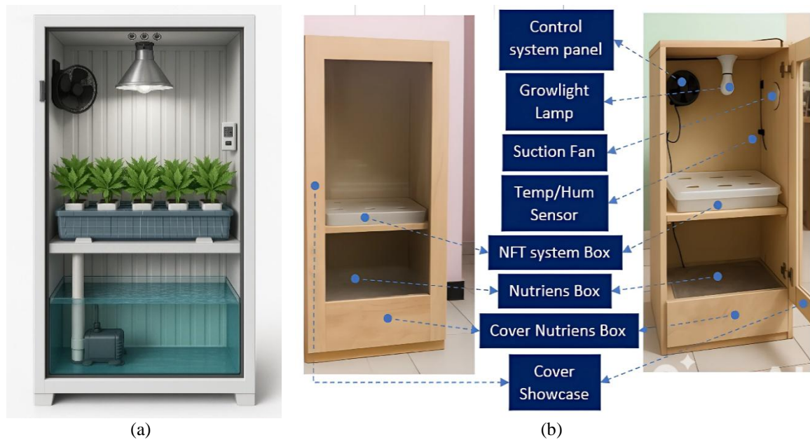
Figure 4. Hydroponic smart showcase prototype; (a) 3D sketch design and (b) showcase front side and inner side
