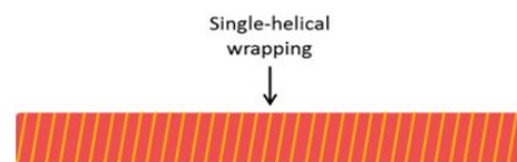
Figure 6. Fiber-reinforced design for twisting and extending motions
