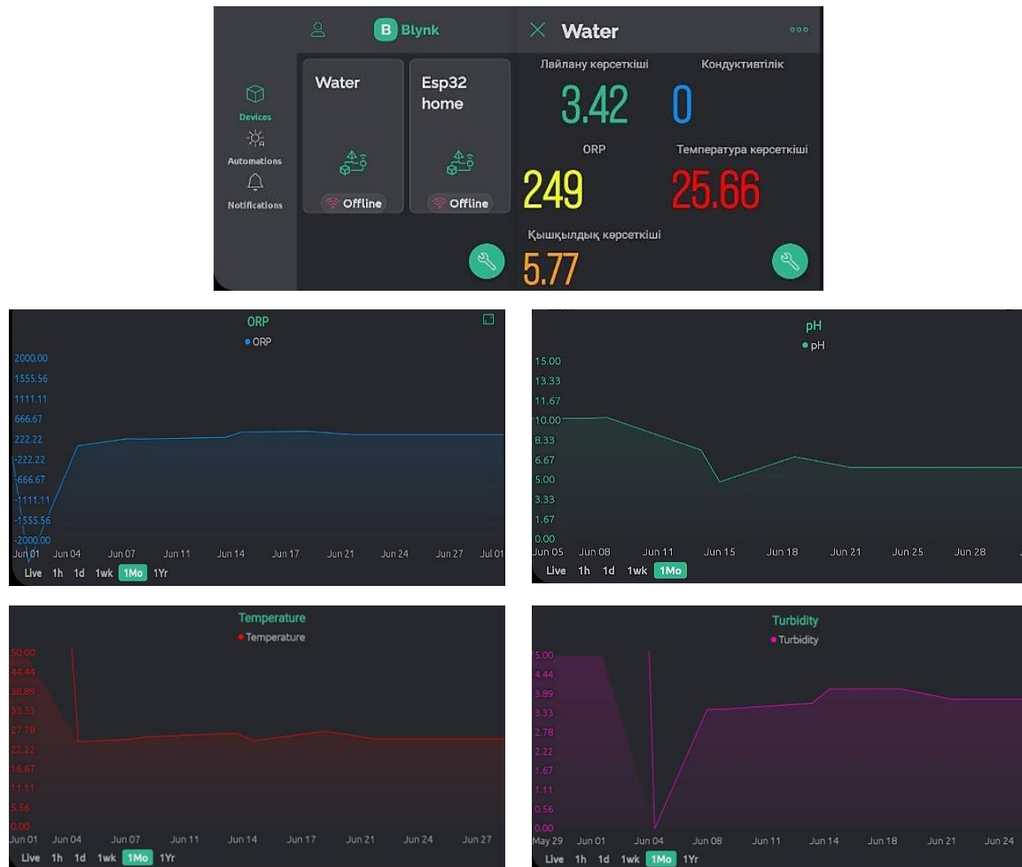
Figure 13. Mobile application Blynk IoT mobile and data changes for one month in stationary mode
