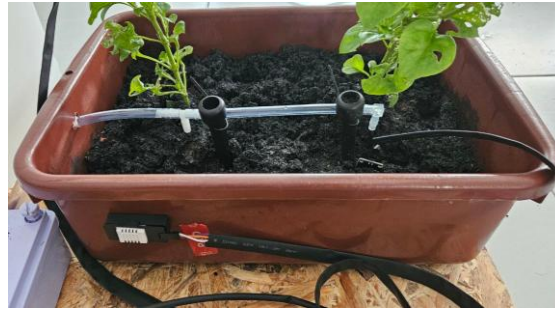
Figure 6. Temperature and humidity sensor on plant crop
