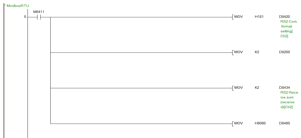
Figure 10. Ladder diagram for setting the PLC as a Slave
